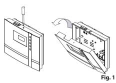
Remove the control device cover. In order to do this loosen the screw at the top of the housing and pull the housing top upward while swivelling (Fig. 1).
